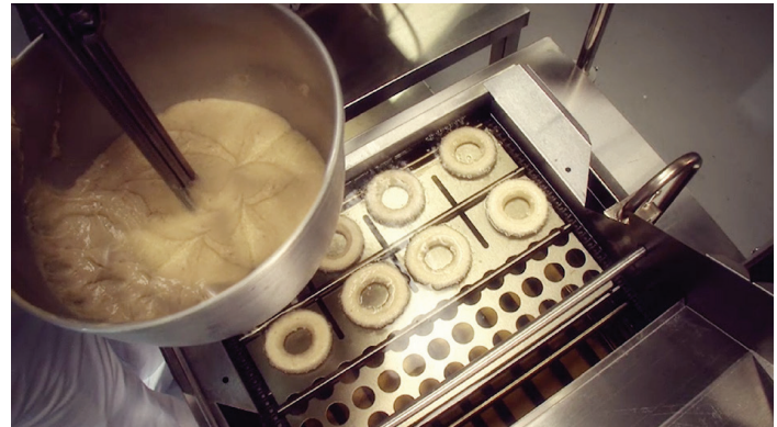
Mark VI Standard with Type F Depositor
